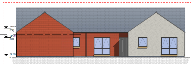
6 HT4.V Proposed Alternative Front Elevation (red brick) 1:50
